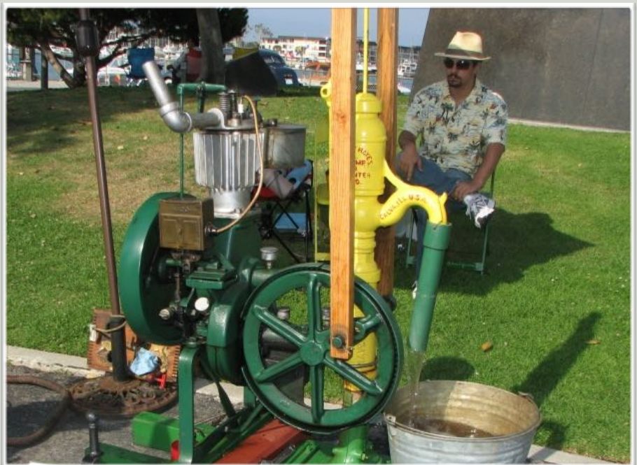
Fuller & Johnson pumping engine shown by Jim Davis. Picture by Larry Evans.
