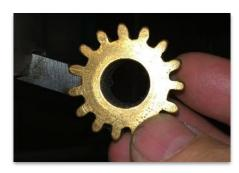
Holding the plastic "gear blank" on the milling machine was done with an indexing head. An arbor was made to fit the inside diameter of the gear blank, with a screw on the end that would hold the blank securely. The indexing head would allow the
