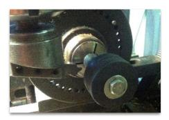
The cutting tool was held in a flycutter. For each tooth of the gear, the cut was made in one pass.
