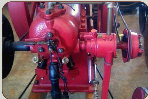
Close up and patent drawing of Hagan's unique rocker arm mechanism
